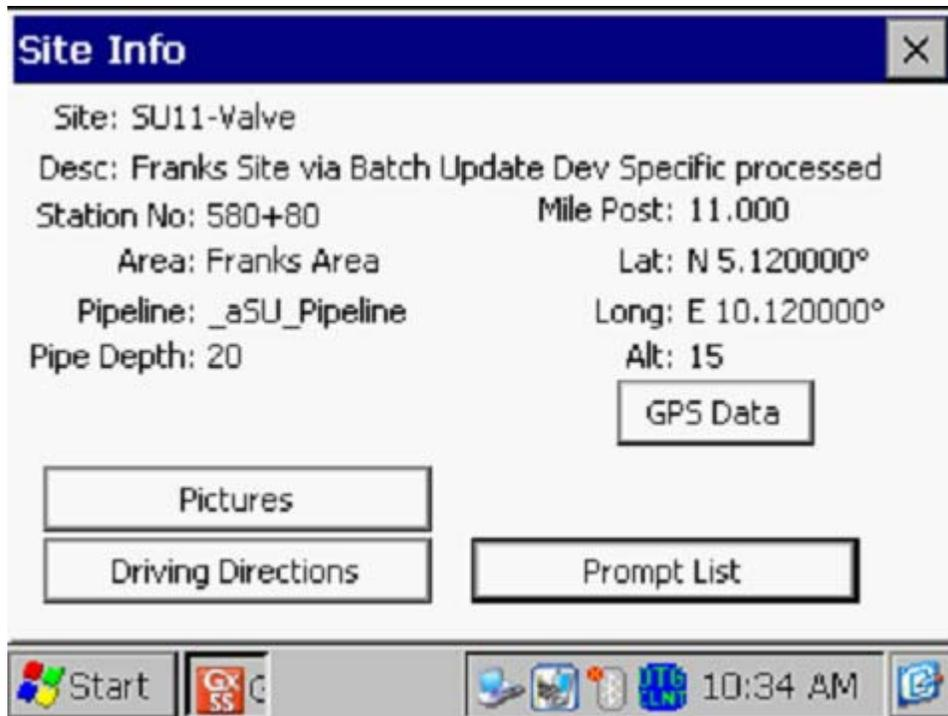
As can be seen from the above screen, important information about the “Valve” test site is displayed. This information about a particular test site was established on the ProActive side and it is downloaded to your Gx data-logger as part of the route data file.
