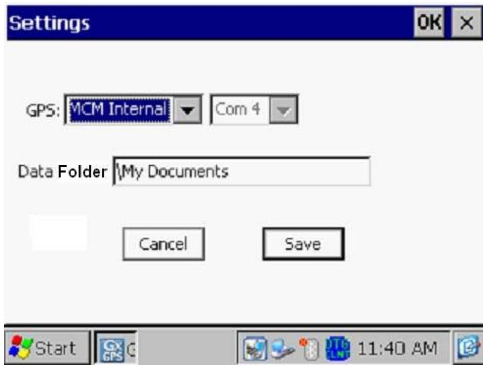
By tapping on the menu button in the GPS field, you can select the type of GPS receiver you are using. You can select either the “MCM Internal” receiver (if you plan to use the built-in GPS receiver on the Gx) or, an external “NMEA” compatible receiver (if you plan to use an externally-connected GPS receiver).
