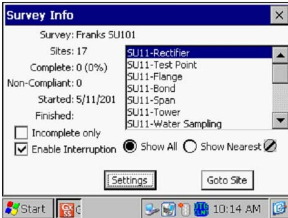
As can be seen on the above “Survey Info” screen, our example route contains 17 test sites and the types of sites are listed on the window. All 17 sites can be viewed using the scroll bar on the right-hand-side of the window.
